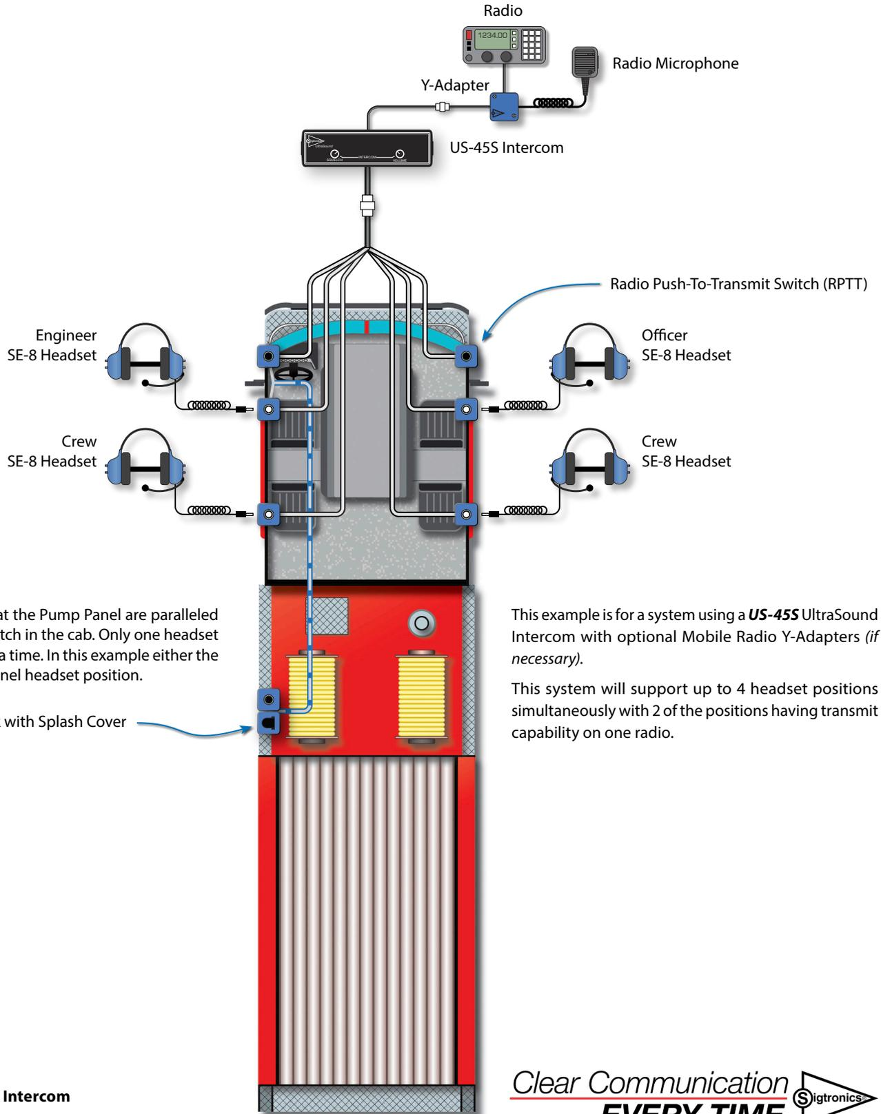
The jack and switch at the Pump Panel are paralleled with the jack and switch in the cab. Only one headset can be plugged in at a time. In this example either the Engineer or Pump Panel headset position.
