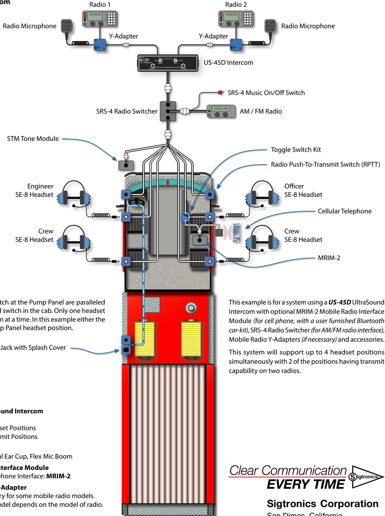
The jack and switch at the Pump Panel are paralleled with the jack and switch in the cab. Only one headset can be plugged in at a time. In this example either the Engineer or Pump Panel headset position.
