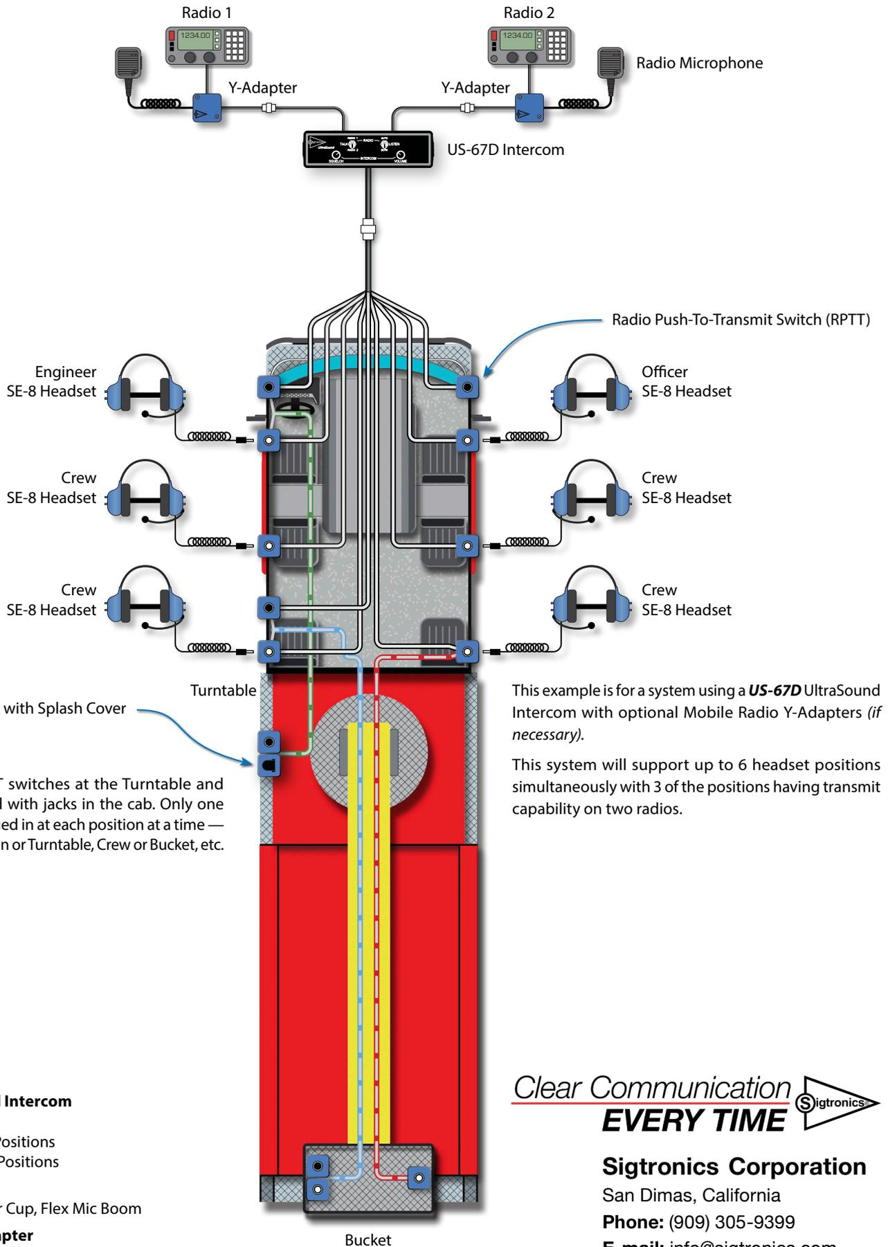
Jacks and Radio PTT switches at the Turntable and Bucket are paralleled with jacks in the cab. Only one headset can be plugged in at each position at a time — either at Driver position or Turntable, Crew or Bucket, etc.
