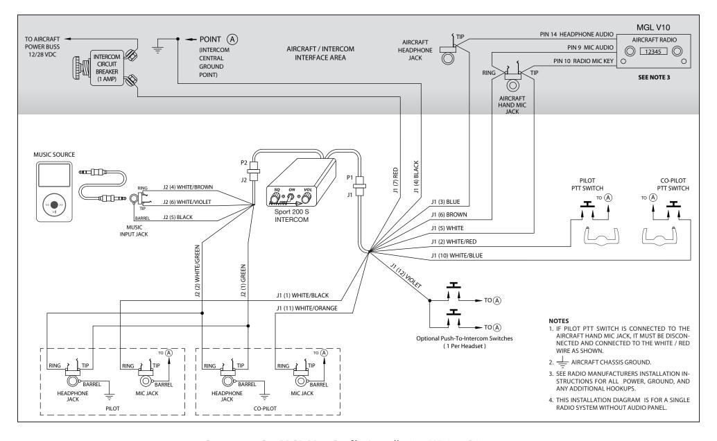
Sport 200S – MGL V10 Radio Installation Wiring Diagram
