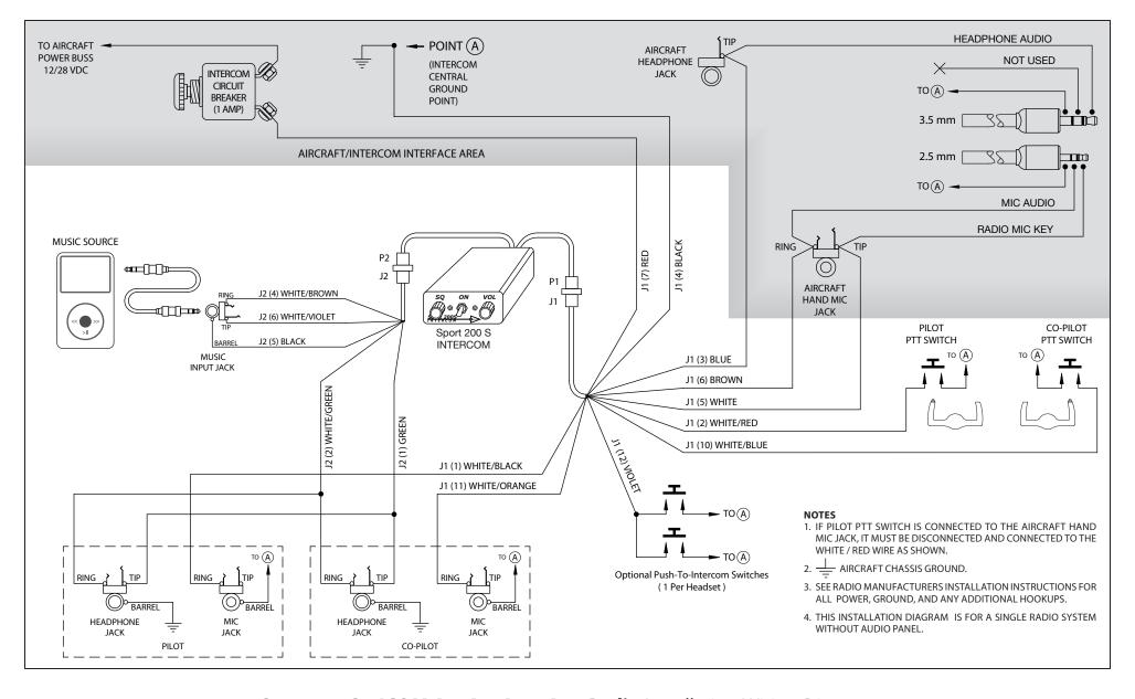
Sport 2005 – ICOM A3, A6, A22, A24 Radio Installation Wiring Diagram
